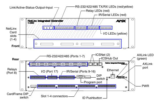
FIG. 6 NI-4000 front and rear panel components
